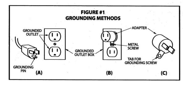
**EXTENSION CORDS** - If it is necessary to use an extension cord, use only a 3-wire extension cord that has a three-blade grounding plug, and a 3-slot receptacle that will accept the plug on the product. Make certain your extension cord is in good condition. Make certain your extension cord wire size is not less that 18 gauge for 25 feet, 16 gauge for 50 feet, and 14 gauge for 100 feet.
